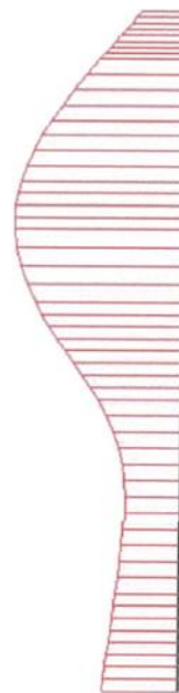
Horizontal displacements (Ux) Extreme Ux -20.39 \times 10^{-3} m
