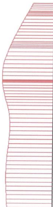
Horizontal displacements ( U_x ) Extreme U_x -39.44 \times 10^{-3} m
